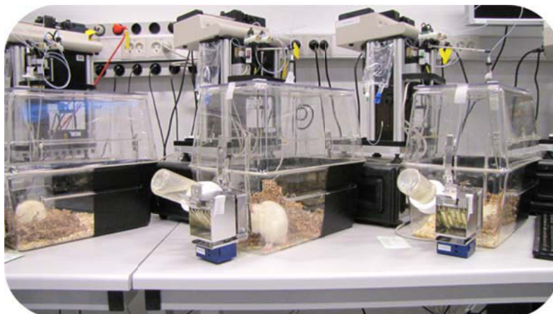
Illustration 9. An illustration of the Accusampler setup. Animals were able to move freely and have free access to food and water during the complete experimentation period.
